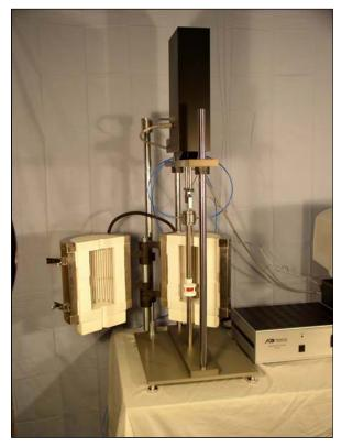
Researchers at The Ohio State University use a TestResources dual column 100R PC Controlled test system to perform tests at low forces. The modular actuator includes a position encoder (0.007 micron resolution) that enables slow constant rate of loading and position control. The system includes furnace and high temperature extensometry for strain control.
