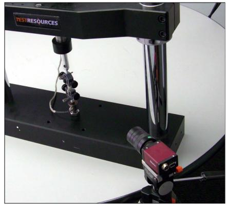
VE23 measures displacements and strains from 500 microstrain to 500% strain and above, for specimen sizes ranging from smaller than 1 mm to very large samples. Strain measurement accuracy is typically better than 0.02%. Setup is simple and requires only an applied random speckle pattern on the specimen. No special illumination or lasers are required.
