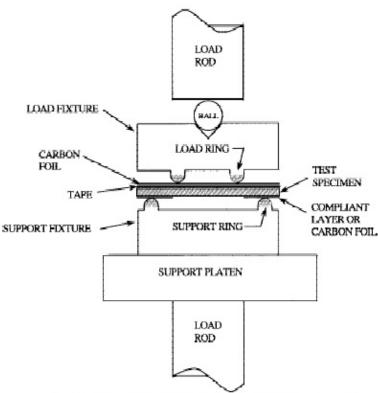
Section View of Basic Fixturing and Test Specimen for Equibiaxial Testing
