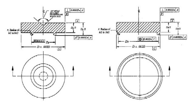
Note—0.4 to 0.8  $\mu m$  surface finish. Harden to 40 Rc or greater. FIG. 2 Load and Support Fixture Designs for Equibiaxial Testing
