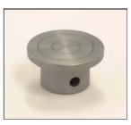
G23 Compression Platens – stainless steel - available in many sizes. (56 mm diameter shown)
