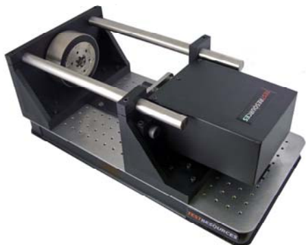
530 Series - Miniature Axial Torsion System for low force dynamic testing - vertical & horizontal mounting.
