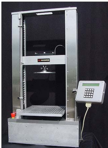
Dual Column 2000M Universal Test Frame with IFD fixtures
