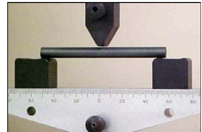
TestResources G238 Bend Fixtures testing ferrite rods.
