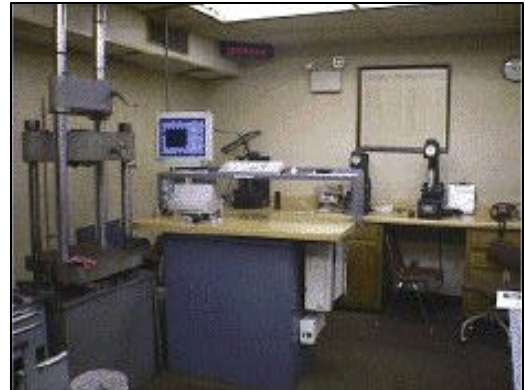
MTest starts by replacing your load indicator and XY Plotter with a PC.
